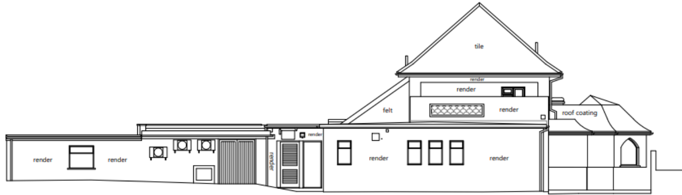
Existing East Elevation
